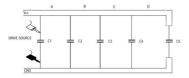
Figure 4-9 Isolation of Open Circuit Decoupling Capacitor
