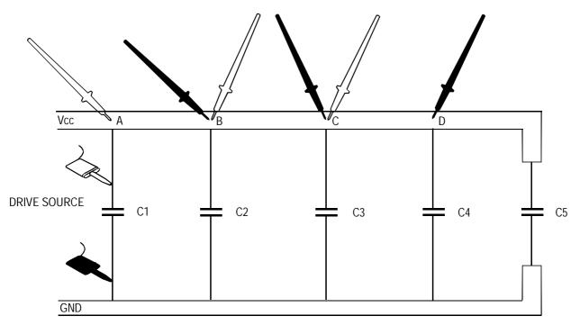
Figure 4-10 Use of Track Voltage Measurement
