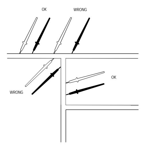
Positive current flowing through the track provides a tone and meter indication of the current flow. Negative current will produce a zero reading, no tone and the PROBES REVERSED LED will light.
