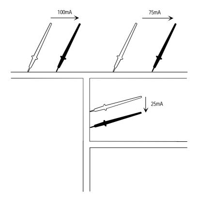
Figure 4-3 Track Current Measurement
